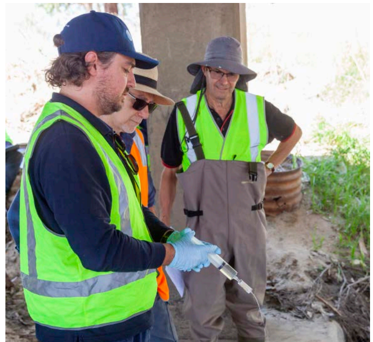
Will Honybun from NCCMA demonstrates using a syringe to push water through the eDNA collection filter. Photo: Greg Martin
